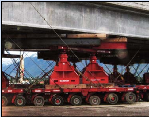
SELF-PROPELLED: Equipment, similar to what is pictured above, will transport and lift the pedestrian bridges into place. Photo courtesy of Mammoet
