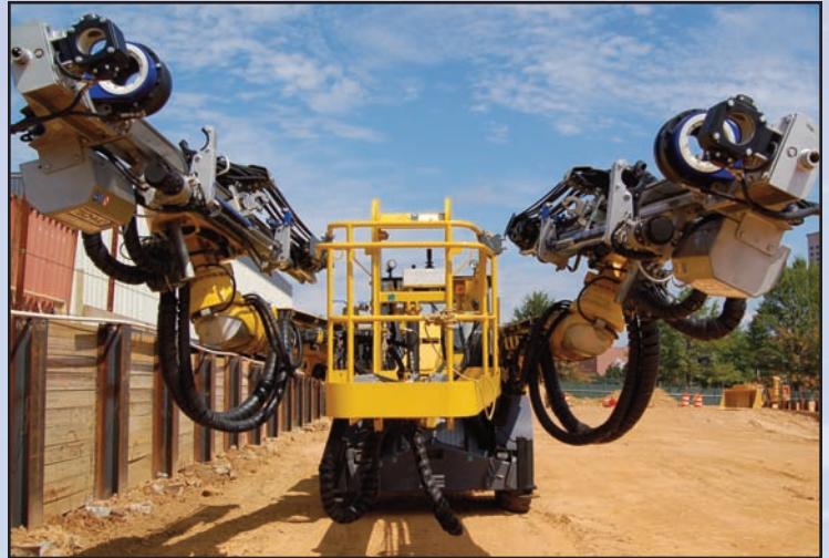
The Drill Jumbo is a specialized piece of tunneling equipment. Photo by Dulles Corridor Metrorail Project
